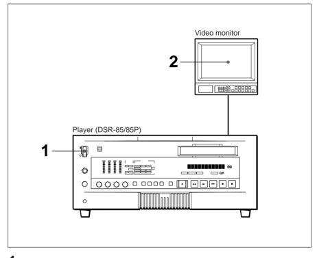
**1** Power on this unit by pressing on the "**I**" side of the POWER switch.
